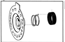
Insert the spring end that is bent inward bearing hole, and the spring end that is bent outward into the spring holder.
