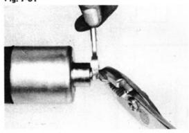
Adjust if necessary after loosening lock nut.
