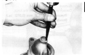
(6) Clean the bore, and install new bushing cover and stake the housing at four positions.
