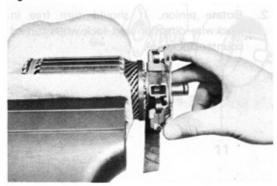
If brush is replaced, dress it with emery cloth to provide proper contact.
